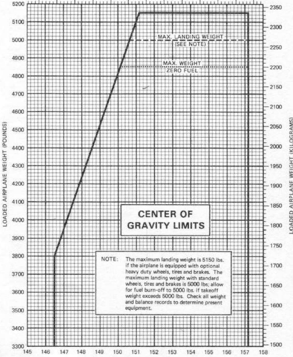
**NOTE:** The maximum landing weight is 5150 lbs. if the airplane is equipped with optional heavy duty wheels, tires and brakes. The maximum landing weight with standard wheels, tires and brakes is 5000 lbs; allow for fuel burn-off to 5000 lbs. if takeoff weight exceeds 5000 lbs. Check all weight and balance records to determine present equipment.
